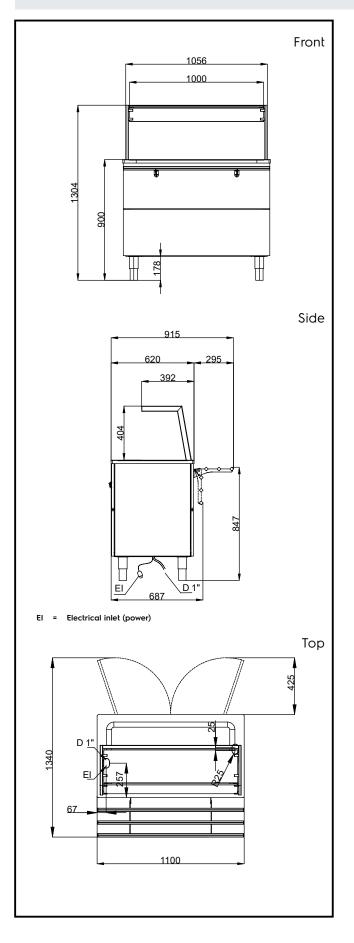
Flexy Compact Refrigerated stainless steel surface on cupboard (3GN) with overshelf with LED lights, H=900mm The company reserves the right to make modifications to the products without prior notice. All information correct at time of printing.
